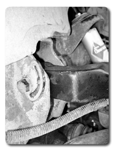
13. Adjust the cams so that both cams are centered. This is NOT the final alignment settings, but is a good start of where they should be. Snug the cam bolts, but do not torque at this time. Check for clearance to the factory pockets and adjust (form / grind) the pocket as necessary to gain clearance. Fig 19
